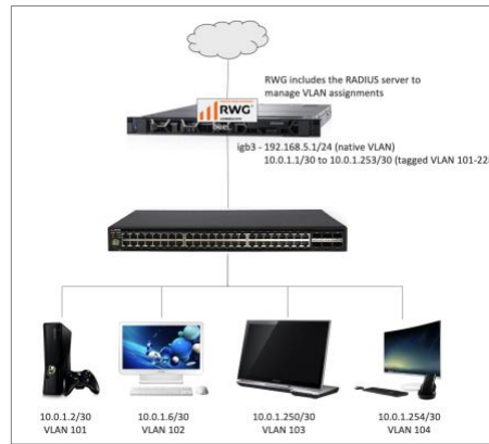
FIGURE 16 – WIRED DEVICES MICROSEGMENTATION USING DYNAMIC VLANS
